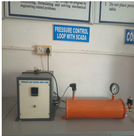
PRESSURE CONTROL LOOP WITH SCADA
