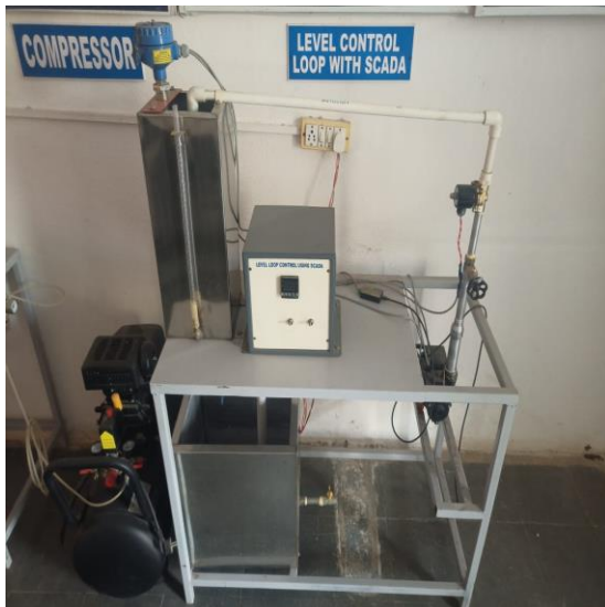
LEVEL CONTROL LOOP WITH SCADA
